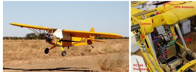
Fig. 1. The autonomous UAV, based on a J3 Cub 1/3 scale model. Sensor payload includes IMU, GPS receiver, downward pointing monocular camera and a PC104 stack.
