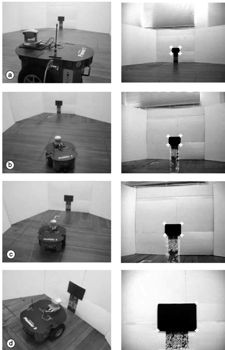
Fig. 18. Snapshots of the docking process for  $\theta_d = 0^\circ$ .
