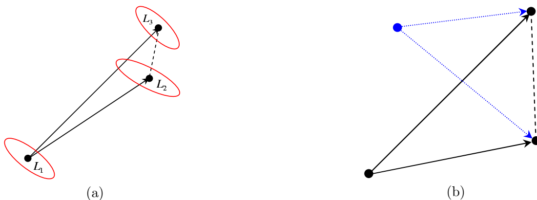
Figure 3.10: Figure (a) shows a LTR which is not geographically well conditioned: the region could flip over. The dots represent the base landmark positions and the ellipses the uncertainty bounds. Figure (b) illustrates a case where two LTRs overlapped.
