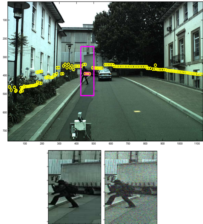
Fig. 7 Perturbation of the visual sensor. Additive random noise is applied to each of the RGB channels in the ROI images, as shown on the bottom images for the ROI corresponding to the detected pedestrian.
