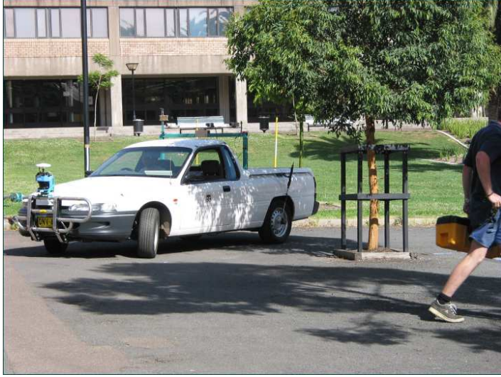
Figure A.1: The utility car used for the experiments is equipped with Sick lasers range and bearing sensor, linear variable differential transformer sensor for the steering mechanism, back wheel velocity encoder and inertial unit.
