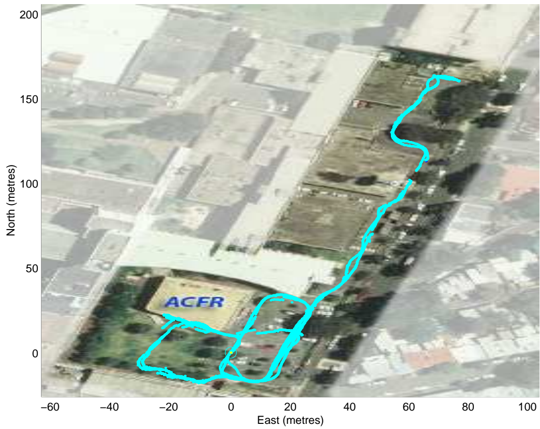
Figure 3.19: Satellite picture of the environment with the trajectory reported from the GPS.
