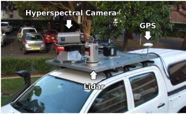
Fig. 8. Setup used to collect ACFR data
