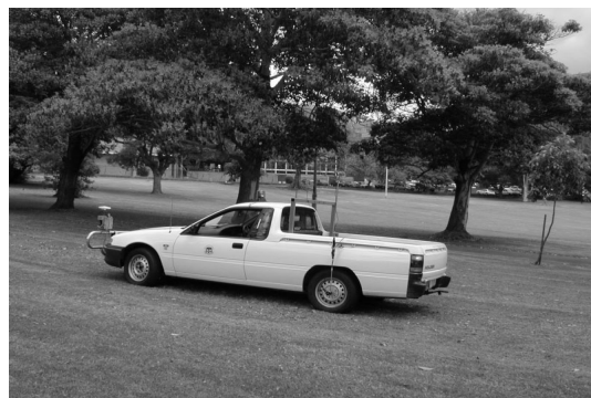
Fig. 4. Victoria Park. The utility car used for this experiment is equipped with a Sick laser range and bearing sensor, linear variable differential transformer sensor for the steering and back wheel velocity encoder.
