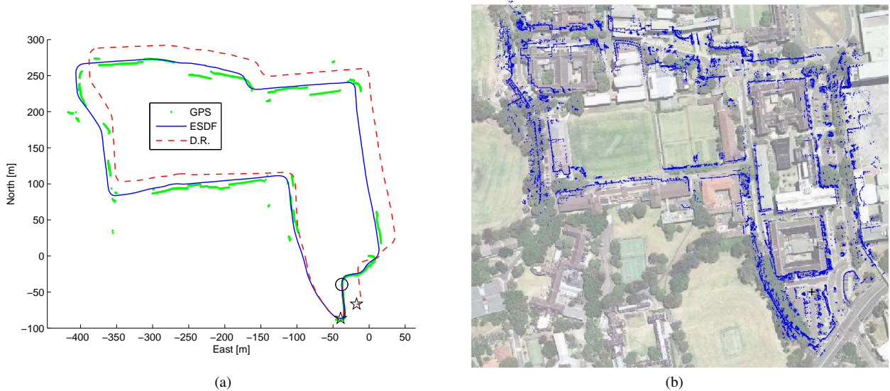
Fig. 6. (a) Estimated vehicle trajectory, GPS and dead reckoning. The ring marks the starting point, the stars mark the end points. (b) Lasermap overlaid on an aerial photograph. Each laser scan was transformed to its respective pose and plotted on top of the photograph.
