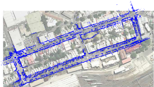
(d) Resulting SLAM map overlaid onto an aerial photograph.
