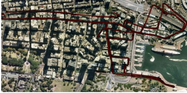
Fig. 4. Vehicle trajectory estimated by our GPS-IMU system, superimposed on an aerial image (rotated 90 deg. clockwise to reduce space). The total trajectory is 9.95 km long. The largest accumulated uncertainty occurs on the top-right part, where the vehicle estimated position possesses almost 200 metres of error. GPS visibility is extremely low in this area of the city.
