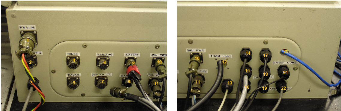
Figure 5.4: External connections to weatherproof box. [Need a single photo that captures entire length.]
