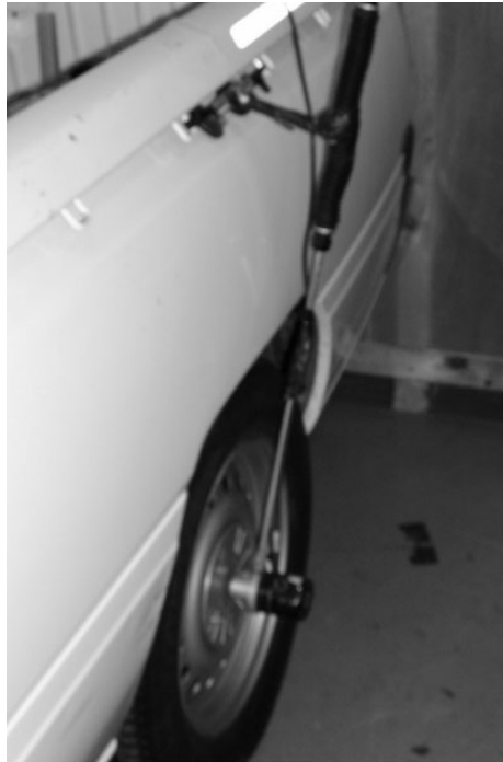
Figure 4.5: The wheel encoder is attached to the left rear wheel-hub.
