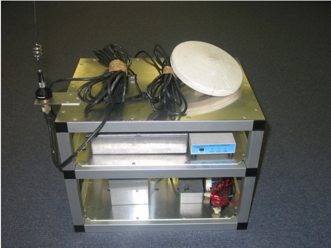
Figure 4.6: GPS Base Station Box.
