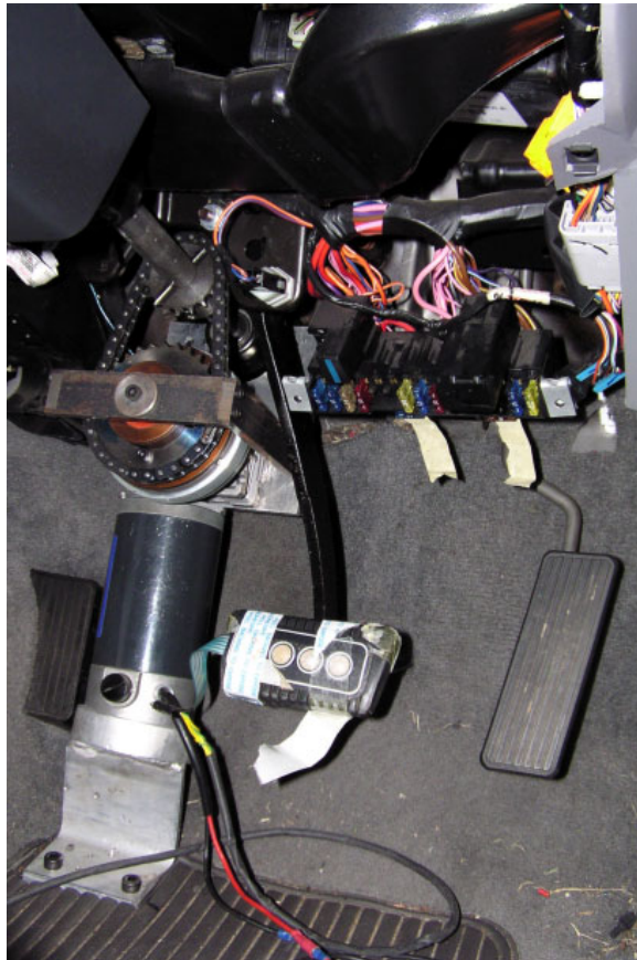
Figure 5.7: Inside cab, driver's side. View steering actuator and manual override pad taped to brake pedal.
