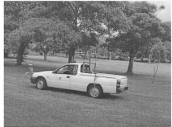
Fig. 7. The utility car used for the experiments is equipped with a Sick laser range and bearing sensor, linear variable differential transformer sensor for the steering and back wheel velocity encoders.
