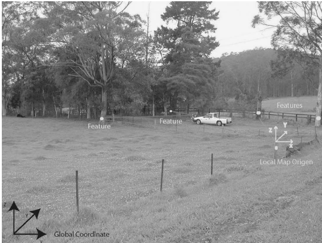
Fig. 1. Navigation using SLAM. The vehicle builds a relative local map and localizes within this map using dead reckoning information and relative observations of features in the environment. The accuracy of the map is a function of the accuracy of the local map origin and the quality of the kinematics model and relative observations. The local map can be registered to the global map if absolute information becomes available, such as the observation of a beacon at a known position or GPS position information.
