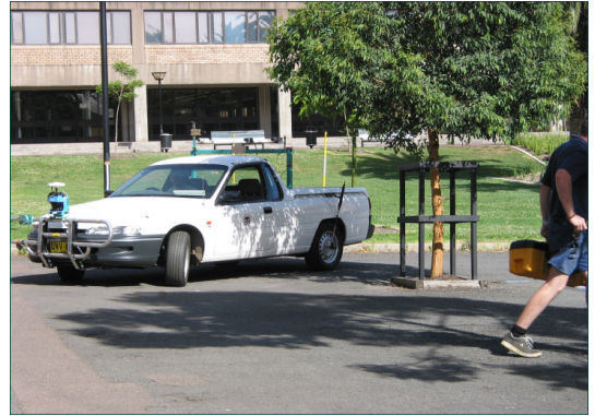
Figure 6: The utility car used for the experiments is equipped with a Sick laser range and bearing sensor, linear variable differential transformer sensor for the steering mechanism and back wheel velocity encoder.
