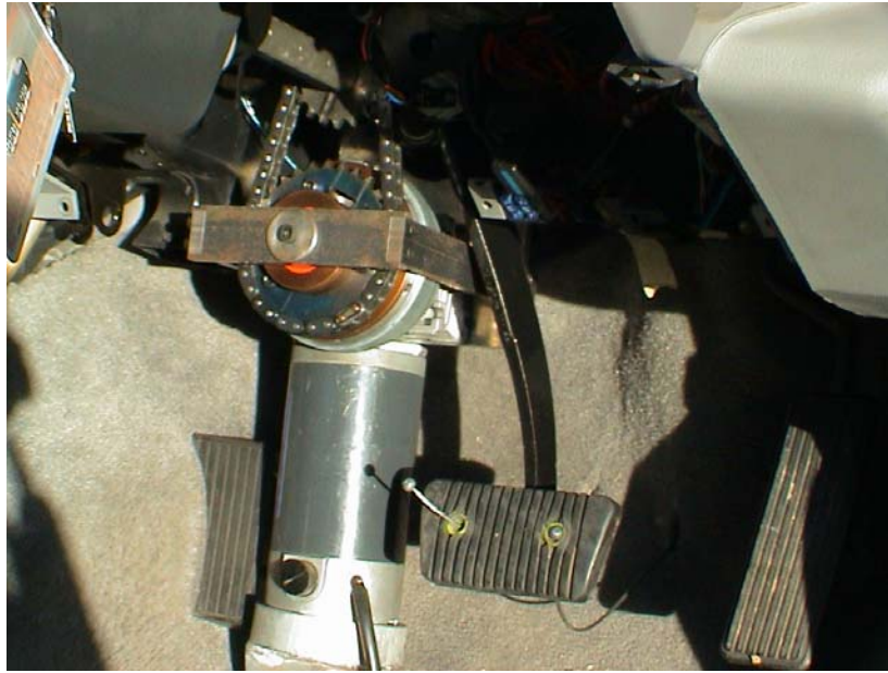
Figure 1.2: Steering control motor and clutch
