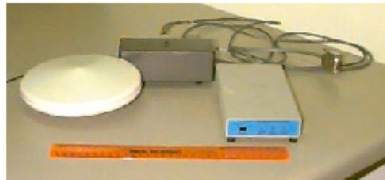
Figure 1.2: The Differential GPS unit for the Ute
