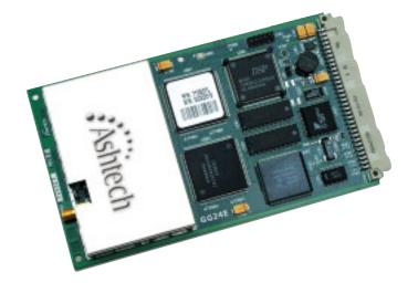
areas where much of the sky and many of the satellites can be blocked. To take advantage of the increased satellite availability, the GG24 from Thales Navigation has 12 channels for L1 GPS and 12 channels for L1 GLONASS, providing all-in-view tracking for both constellations.
