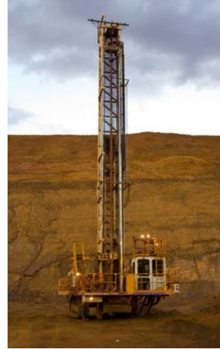
Figure 2. Terex Reedrill SKSS-15 drill rig, used to collect data for the experiments.
