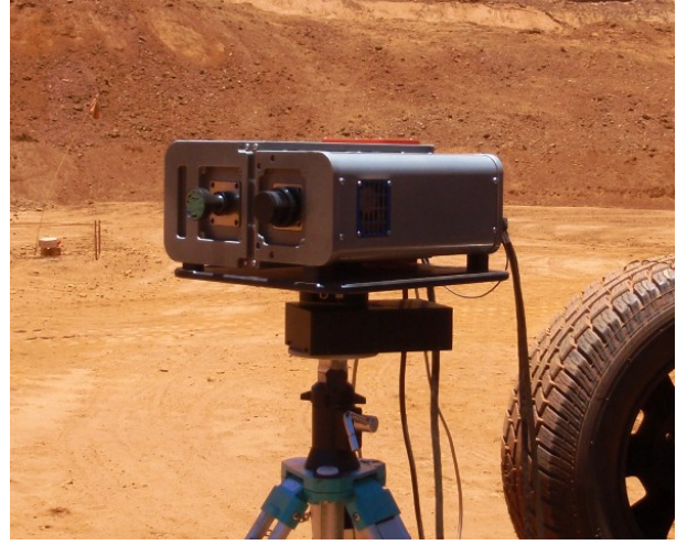
Fig. 1. Hyperspectral camera used to acquire data for the experiments; note that there are two sensors, one for the VNIR and other for the SWIR.
