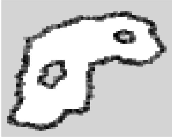
Figure 2.1: Occupancy grid map. The probability of occupancy for each grid square is defined by a value bounded by  $(0, 1)$  such that 0 indicates definitely not occupied (free space) and 1 means definitely occupied. A prior probability of 0.5 implies unexplored space (depicted by the light gray regions). Note that the rectangular grid is not an efficient representation of non-rectangular environments such as this one.
