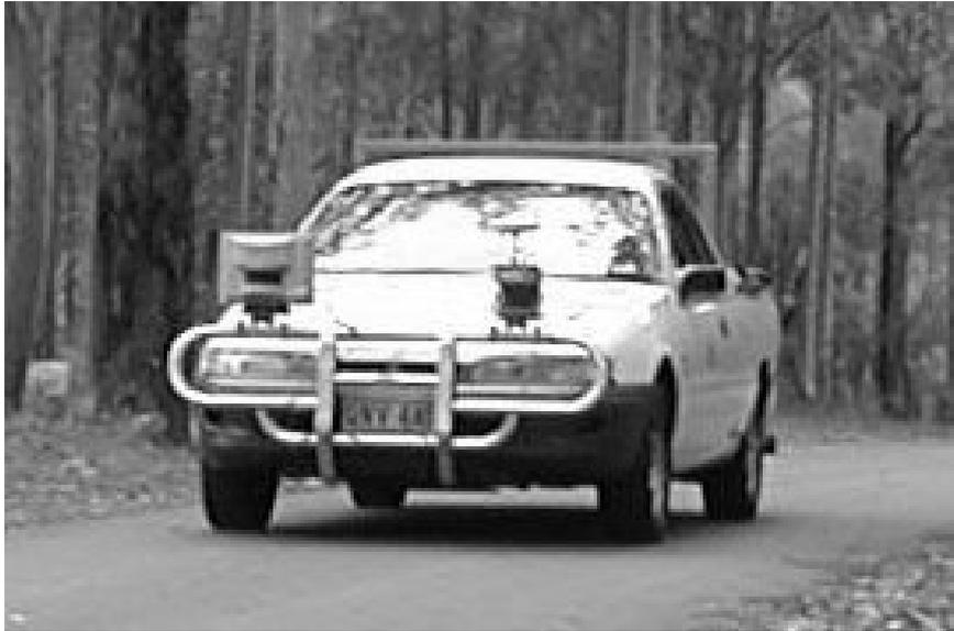
Figure 2.7: Two scanning lasers (different models) attached to the front bumper of a standard utility vehicle.
