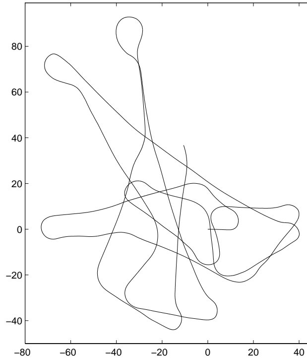
Fig. 10. Encoder dead reckoning. Unmodelled properties of the vehicle motion, such as wheel slip and non-linear parameters, contribute to rapid deterioration in the odometric pose estimate.
