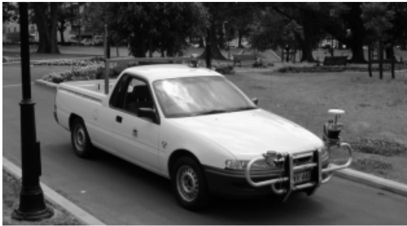
Fig. 3. Utility vehicle with laser sensor in park environment.
